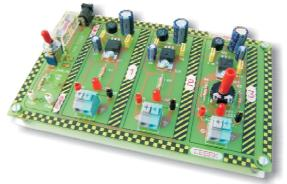
The Edu-009 practice describes the process to convert the alternate current form the mains into a discontinued voltage, using fix and variable voltage regulators. Applying the 78XX and LM317 family, in three practices you can see different parameters required by the power supply for the regulation process. An original instruction manual from manufacturers is included, to allow the student to familiarize with control parameters and these components' design.
