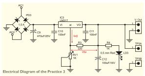
As concern the design of the regulator's part, in a fix or variable power supply, you have to maintain two disconnection capacitors at the entrance and the exit of the transformer. Both are necessary to avoid the inductance caused by the capacitive filter. In the practice C10 and C11 offer this function. Normally, its value is 100nF, although if some manufacturers advise to use a 220nF capacitor at the entrance.
