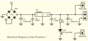
Apply the channel N°1 of the oscilloscope between the 7805's input pin and the central one, (ground). The channel 2has to be applied between the point test TP1 or TP2 according to the practice. The oscilloscope's adjustment will remain in dual visualization, times basis selected in 2 msec, and 0,2V/div AC in the channel N°1 and 5mV/div AC in the channel n°2.
