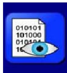
To view the logged data, click on this icon. The logged data will be displayed over the plot area where it can be examined. This same file can be ported to a spread sheet program like Excel for further analysis and plotting. To find the path to the logged data go to **Program Files → Horizon FCA → Data** on your hard disk.
