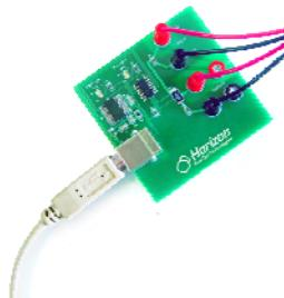
The Data Acquisition Board is the electronic interface between devices such as a fuel cell, solar panel and wind turbine. When connected to a computer via a USB cable, it measures and computes voltage, current, resistance and power then transmits these electrical quantities 3 times a second to the computer. The computer software displays these quantities as both numbers and colored line plots as they are transmitted.
