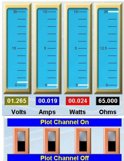
The four meters display the voltage, current, power and resistance. Their scales are fixed and unlike the grid plot area, cannot be changed.
