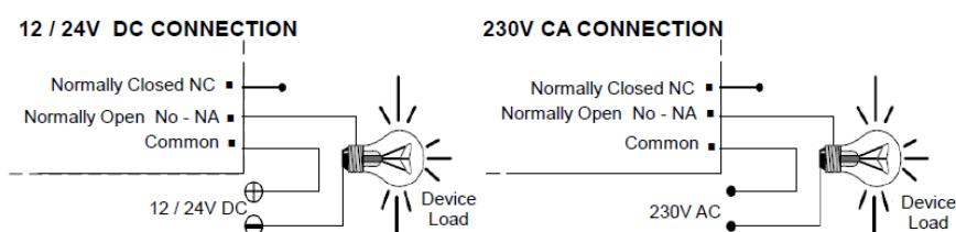
**CONSIDERATIONS ON DEPARTURE.** During the operation of the circuit, and depending on its load, a fluctuation or incorrect operation of the output may occur. If this occurs, install an anti-spark circuit between the two relay contacts used in the connection, as shown in the drawing.
