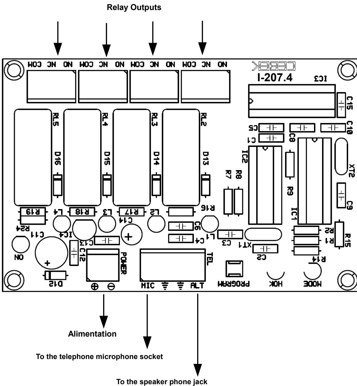
**OUTPUT CONNECTION. BURDEN.** The output is carried out through a relay, a device that accepts any type of load that does not exceed 3 A. The relay has three output terminals. The Normally Open at rest (NO), the Normally Closed at rest (NC), and the Common. The operation of this mechanism is identical to a switch, whose two terminals will be the NA and the Common.
