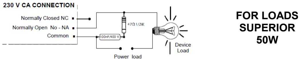
**NOTE :** To connect loads to 12 V. DC, eliminate resistance and put only capacitor
