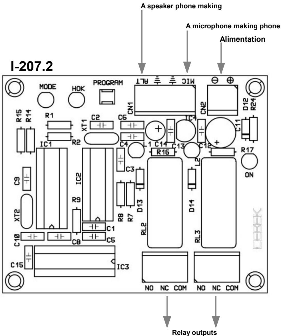
**OUTPUT CONNECTION. LOAD.** The output is controlled by a relay device that supports any type of load does not exceed 3 A. The relay has three output terminals. The rest normally open (NO), the normally closed at rest (NC) and the Joint Operation of this mechanism is identical to a switch, whose two terminals NA and the common
