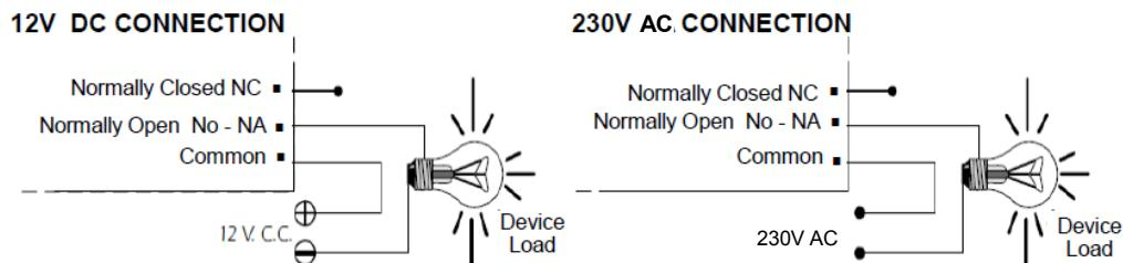
**ABOUT THE OUTPUT.** During operation of the circuit, and according to its load, this could be a fluctuation or an incorrect operation of the output. If this occurs, installing a spark circuit between the two relay contacts used in the connection, as shown in the drawing
