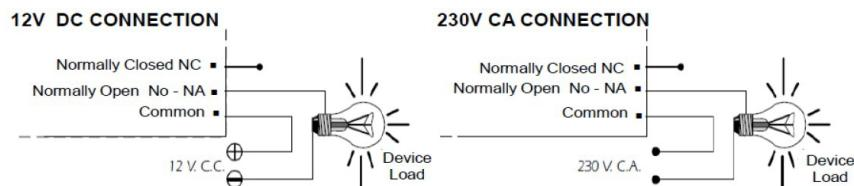
**DEPARTURE CONSIDERATIONS.** During the operation of the circuit, and depending on its load, a fluctuation or incorrect operation of the output may occur. If this happens, install an anti-spark circuit between the two relay contacts used in the connection, as shown in the drawing.
