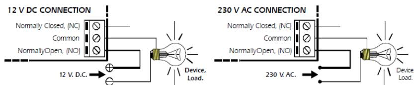
**OUTPUT CONSIDERATIONS :** During the operation of the circuit, and depending on its load, a fluctuation or incorrect operation of the output may occur. If this occurs, install a non-sparking circuit between the two relay contacts used in the connection.
