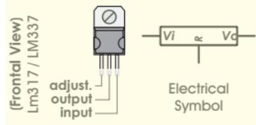
The practice uses a LM317 model, with the same pins number and similar electrical symbol, but with a different pins assignment regarding the 78XX family. Even there is other encapsulated, the indicated one in the drawing is the most common.
