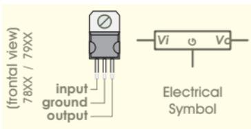
can be positive or negative according to the model. Between positive fix regulators the 78XX family is the highly important, where XX indicates the fix output voltage value. 5V for the 7805, 12V for the 7812, etc....The same type of 79XX family, offer negative voltages.
