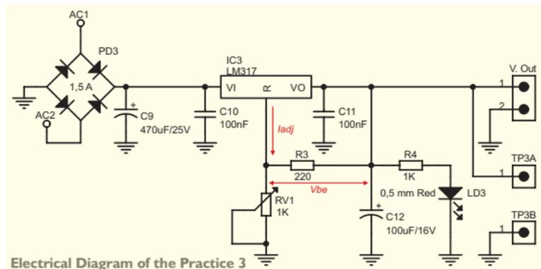
As concern the design of the regulator's part, in a fix or variable power supply, you have to maintain two disconnection capacitors at the entrance and the exit of the transformer. Both are necessary to avoid the inductance caused by the capacitive filter. In the practice C10 and C11 offer this function. Normally, its value is 100nF, although if some manufacturers advise to use a 220nF capacitor at the entrance.
