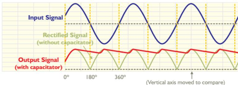
**Capacitive Filter.** The obtained signal after the rectifier bridge is a pushing voltage, far away from a minimally stabilised voltage. Nevertheless, adding the suitable capacitor, because of the component's load-unload, you can avoid that the voltage will reduced under a determined level. Graphically, you can see more clearly that the signal, after the capacitor, is converted into an almost-continuous voltage with the characteristic form of saw teeth.
