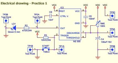
If the B comparator input is inferior to PCI, the comparator output changes and provokes the Reset of the flip-flop which also switch the state of Q at low level. Therefore, Q goes to high level, (output = Vcc and Ld1 is lighted on). With Q at low level, NPN goes to cuts, unblocking the load of C4 through the Time resistor.
