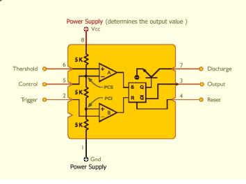
Output. Pin 3 goes to high level during the output impulse.
