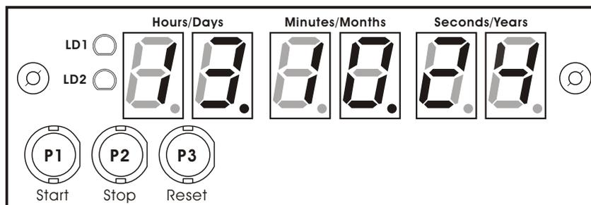
Therefore, till you Stop or Reset the CD-34, the module will daily record operating times of the controlled apparatus or devices during the month. At the end of the month, if you not activate the Reset function, the module automatically reset the module and all data will start from zero. The Stop button is charged to stop the module's timing, and to leave it awaiting for a new information. All registers will be stored on the memory. LD1 led will light off.
