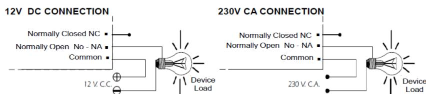
**CONSIDERATIONS ON THE OUTPUT.** During the operation of the circuit, and depending on its load, there may be a fluctuating or incorrect operation of the output. If this occurs, install a non-sparking circuit between the two relay contacts used in the connection, as shown in the drawing.
