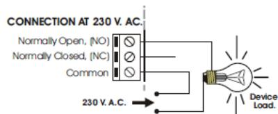
**ABOUT THE OUTPUT:** During operation of the circuit, and according to its load, a fluctuation or an output malfunction may occur. If this happens, install an anti-spark circuit (capacitor and resistor 100nF/400 V. 47. ½ W.), between the two relay contacts used in the connection.
