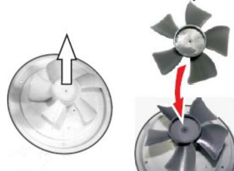
6 - Enter another set of blades, inserting a pressure shaft engine and the position of the image Reassemble the entire set
