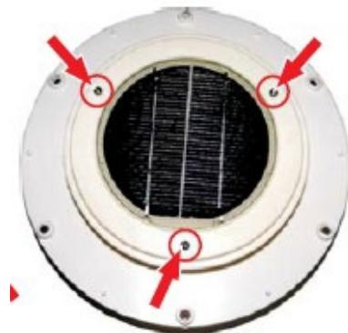
4 - Unscrew the three screws that secure the solar panel. now carefully remove
