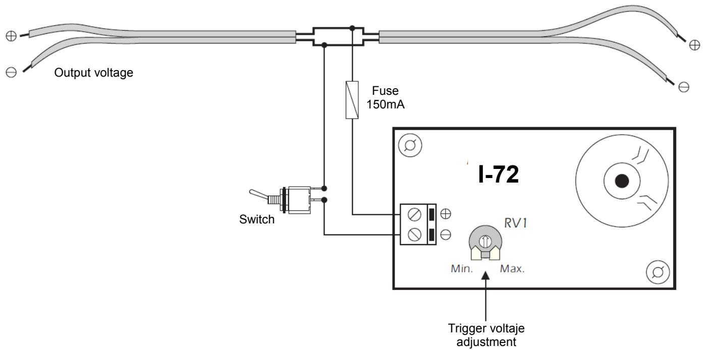
Parallel connection of the module for Making Voltage to Control.
