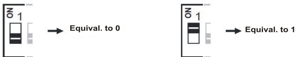
Fig.2 Switches value according to their position
