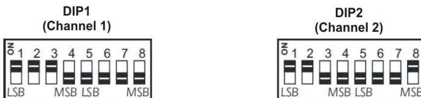
Fig.6 How to configure the channel 1 with the number 7, and the channel 2 with the number 83
