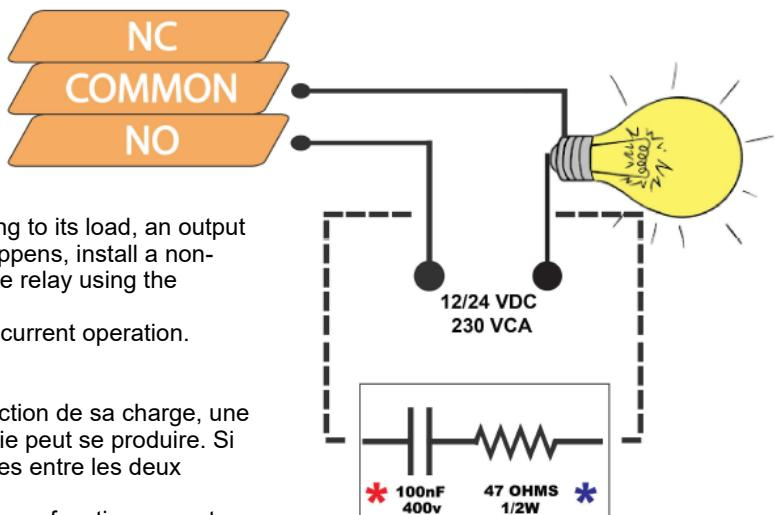
During the operation of the circuit and according to its load, an output fluctuation or malfunction may occur. If this happens, install a non-sparking circuit between the two contacts of the relay using the connection.
