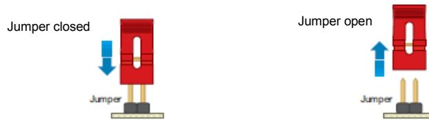
**WORK MODE :** It can work in three ways, as closing one of the corresponding jumpers that configure: In, Out or Static. The closure is unique, so it should always remain open the remaining two
