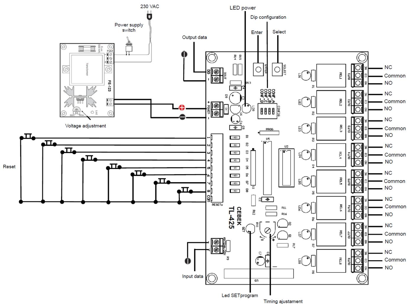
**Factory reset** : Erases the control and setting, turn off the power 10 seconds with enter button and selec pressed simultaneously, turn on the power. Keep tight, the LED program blinks fast for 5 seconds, stays fixed and then off, the receiver is reset .
