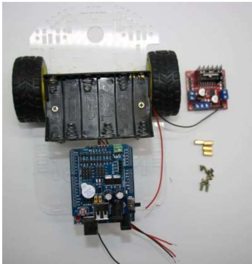
Figure 5- 1 : Pieces that we will use to fix the control circuit of motors
