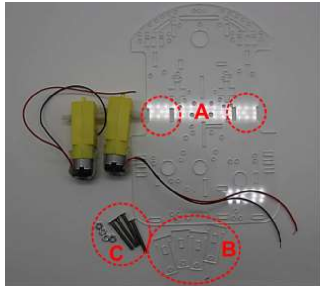
Figure 1 – 4 : Pay attention to motors details in order to place them in the correct position
