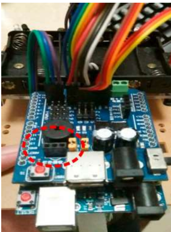
Figure 8 – 3 : Location of the base where the infrared receiver must be connected.
