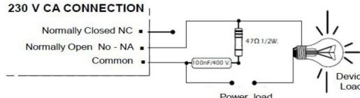
**INSTALLATIONS CONSIDERATIONS:** Do not intalarse humidity places, high and close temperatulas liquids. Perform installation in a vented enclosure.
