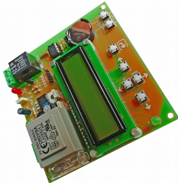
I-520 Weekly programmer to 230VAC I-521 Weekly programmer to 12VDC.
