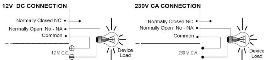
**CONSIDERATIONS ON RELAY:** Especially with inductive loads, a relay output can produce a fluctuation, apportionment, or malfunction. If this happens, install an anti-spark between the two relay contacts used in this connection, that ensure absorption peak current that causes the circuit above problem.
